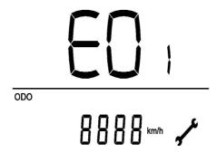
If a fault is detected a spanner will appear in the lower right conrner of the display and the error code will be displayed.
