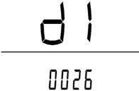
Press **2** button to select the wheel diameter using + and - buttons to adjust the wheel size from 8 to 28 inch, the default value is 26 inch.
