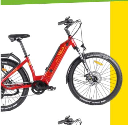
The Tranzit MD is a mid-drive crossover bike, meaning it is equally at home around town and on light trails (if you're looking for a more serious trail bike then look at our Ascent MD). The standard 522 watt-hour battery combined with mid-motor efficiency delivers ample range but can be upgraded to 630 watt-hours for even greater range. Here's what Consumer Reports NZ said about the Tranzit MD:
