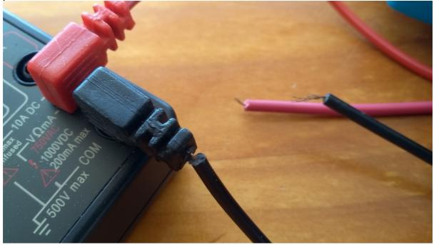
This clearly illustrates one of the main reasons that you shouldn't buy a cheap multimeter. To keep the cost down, cheap materials are used, and this type of failure is common.
