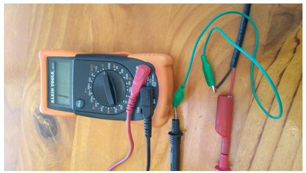
Obviously be aware of any exposed metal carrying voltage when using probes or clip leads, and ensure they cannot touch each other or any conductive component (or the meter user!).
