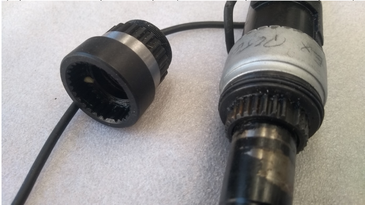
4) Splined hub and torque sensor spline (Note the wide spline in both components)
