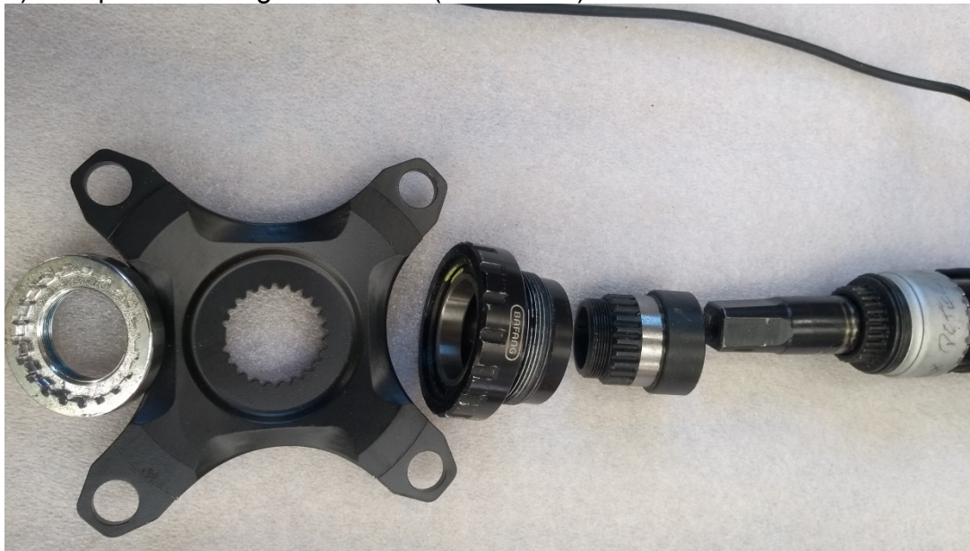
Chromed ring, Chainring hub, bearing housing, splined hub, torque sensor.
